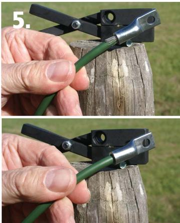
5. Insert the connector with cable into the CRIMP slot and close the tool on it.
