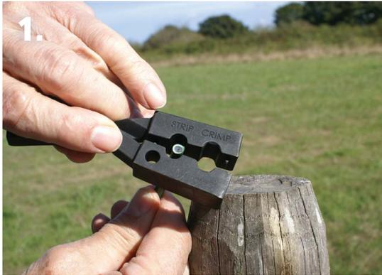
1. Put the end of the cable into the hole marked "strip"
