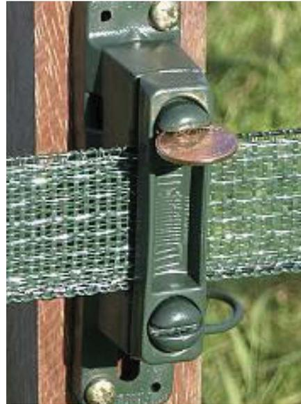
Once the insulator has been attached onto a line post, position the tape, close the cap, and screw the bottom peg in first.
